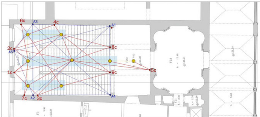
Fig. 6 Reference system with fixed targets for the registration of point clouds
