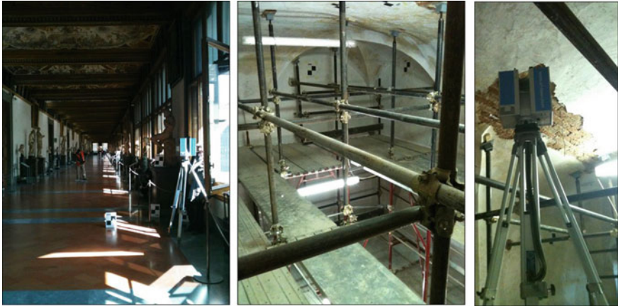
Fig. 1 Laser scanner survey activities in the museum complex of the Uffizi
