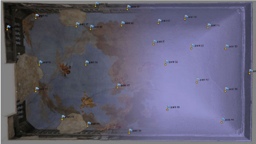
Fig. 11 Oriented by SfM image projection on the laser scanner mesh model
