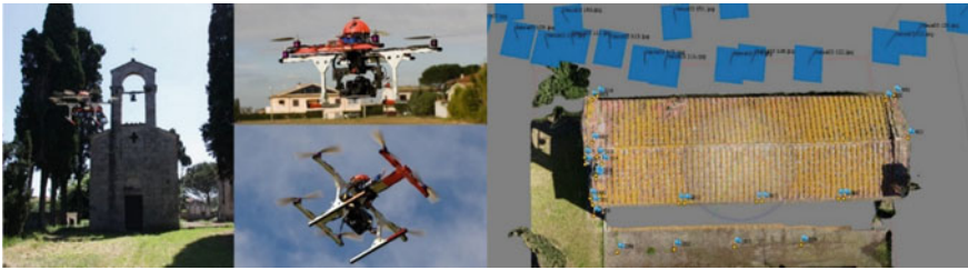
Fig. 15 UAV photogrammetric survey
