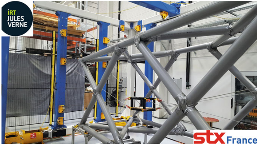
Fig. 2 CAROCA prototype: a reconfigurable cable-driven parallel robot working in a cluttered environment (Courtesy of IRT Jules Verne and STX France)
