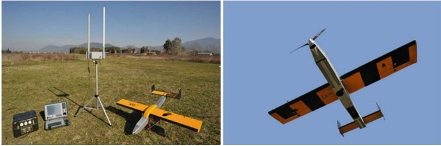
Fig. 1 Fixed-wing UAV for photogrammetric purposes
