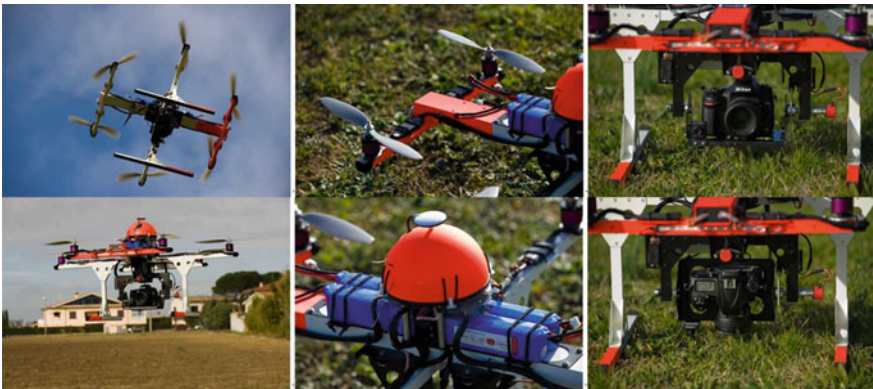
Fig. 2 Rotary-wing UAV for photogrammetric purposes
