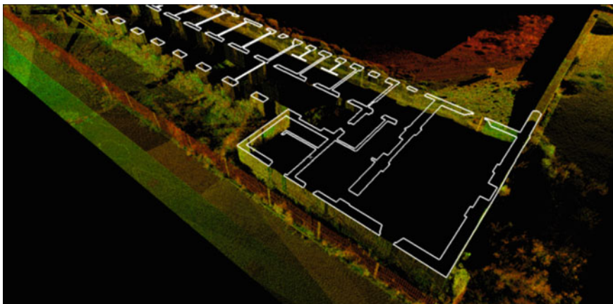
Fig. 5 Integration of laser survey with internal survey retrieved from archival research
