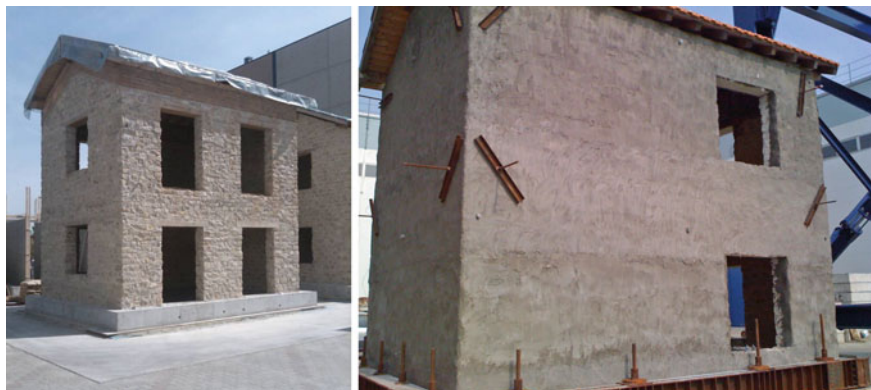
Fig. 5 3D View of the unreinforced (left) and reinforced (right) stone building, Reproduced from [17, 66]
